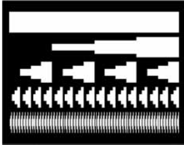
Fig. 3. Mask pattern for quaternary ( q = 4 ) detectors.
