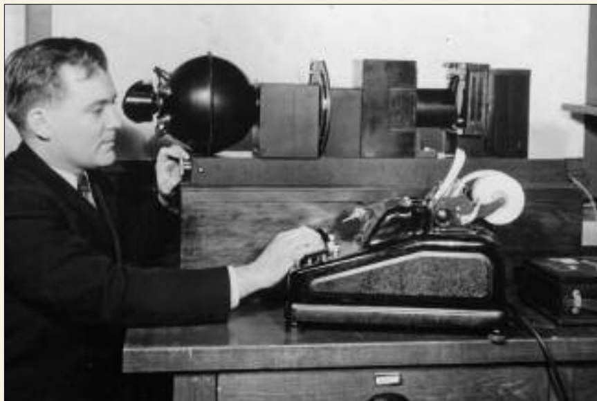
David MacAdam, editor of JOSA from 1964 to 1975, with his colorimeter for the determination of "MacAdam ellipses."
